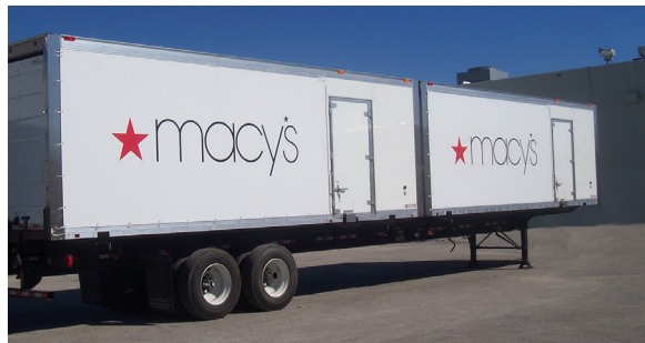
Two demountable bodies on a semi-trailer await the tractor for pick-up. Doors at the front and rear of each body allow multiple bodies to be loaded at one bay.
